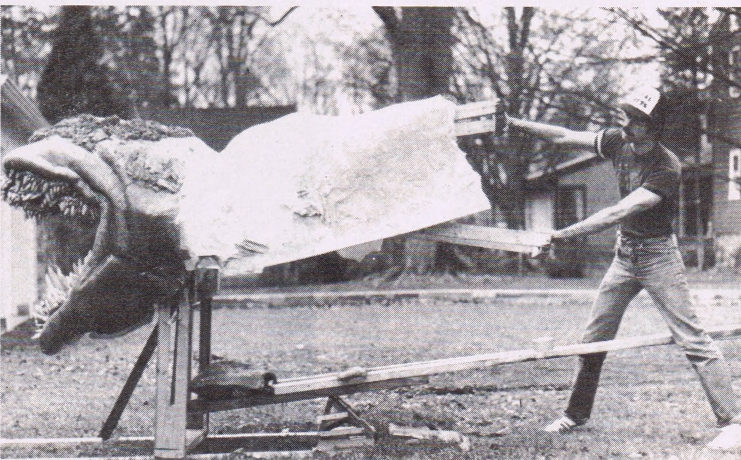
Above: Author John Dods tests the giant “Deadly Spawn” control mechanism, which operates like a giant pair of scissors. Two crew members operated the mechanism during the shot. The bulk of the monster's shape was made of chicken wire covered with foam rubber strips stapled together. The skin was built up with paper toweling covered with latex rubber. This helped to minimize the weight of the monster. Below: Tim Hildebrandt and John Dods confer on the miniature set that they built for The Deadly Spawn .
